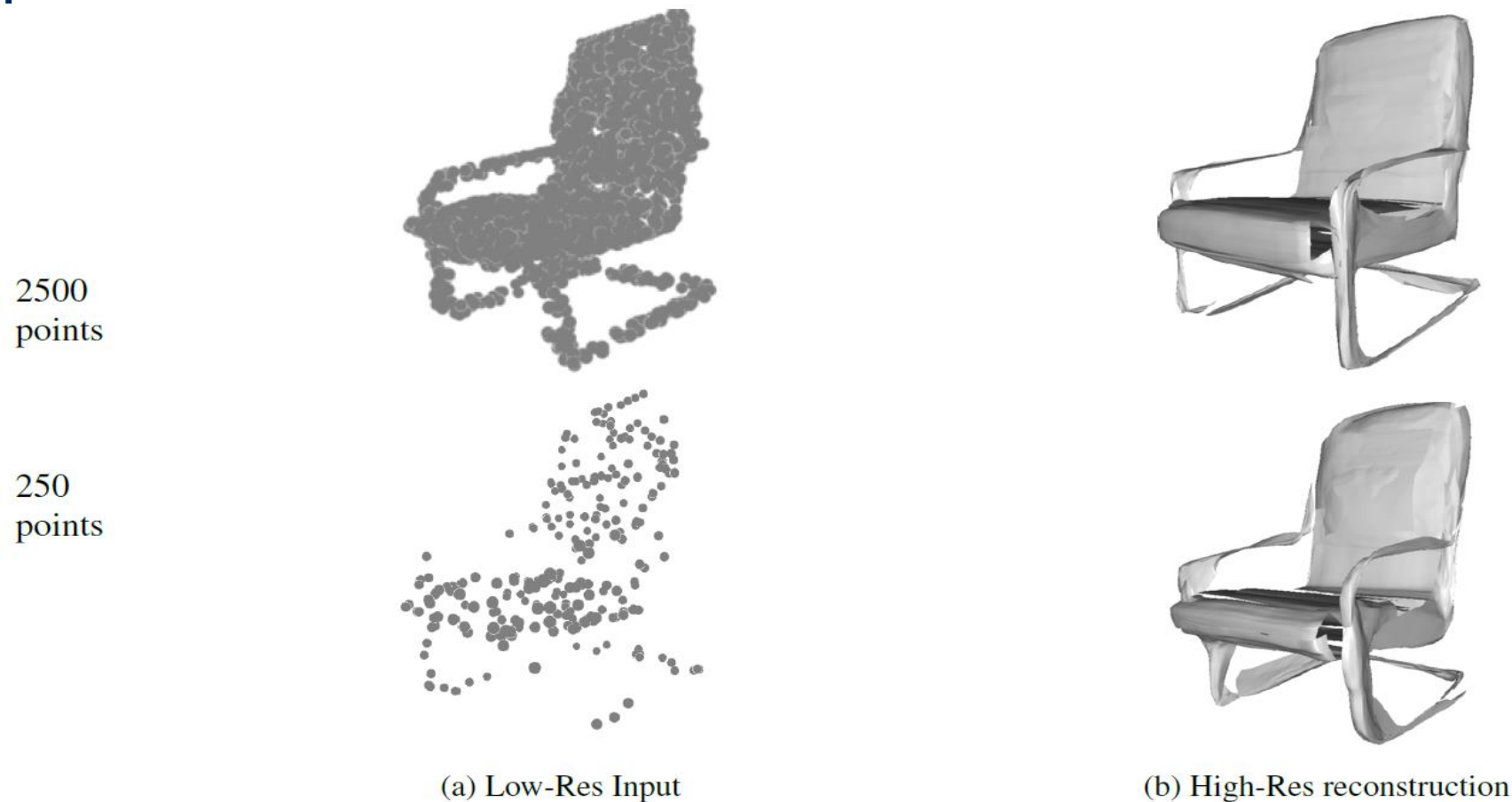
Figure 8. Super resolution. Our approach can generate meshes at arbitrary resolutions, and the pointnet encoder [25] can take pointclouds of varying resolution as input. Given the same shape sampled at the training resolution of 2500, or 10 times less points, we generate high resolution meshes with 122500 vertices. This can be viewed as the 3D equivalent of super-resolution on 2D pixels.
